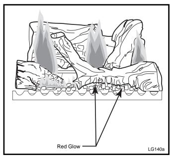
Fig. 52 Correct burner flame pattern.
